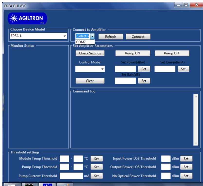
Figure 4: Remote control software: Port selection
